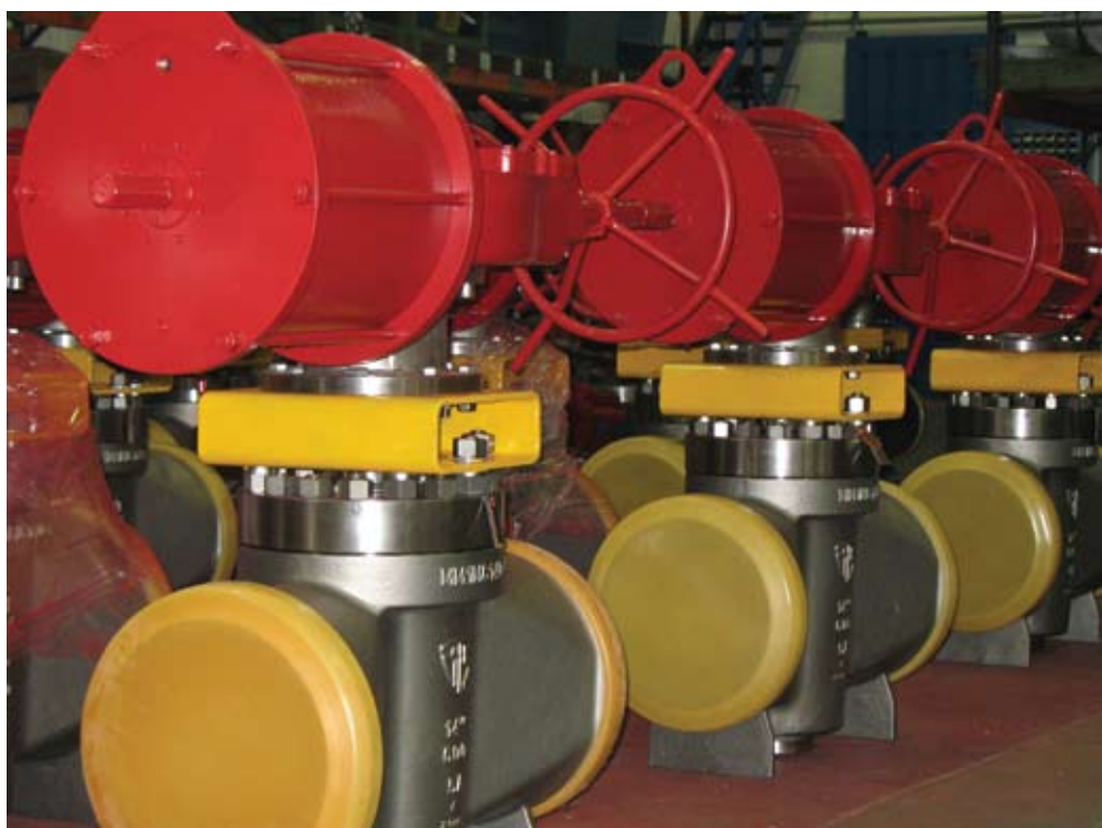
High-pressure plug valves await shipping at an MTS Valves warehouse in the north of Spain.
